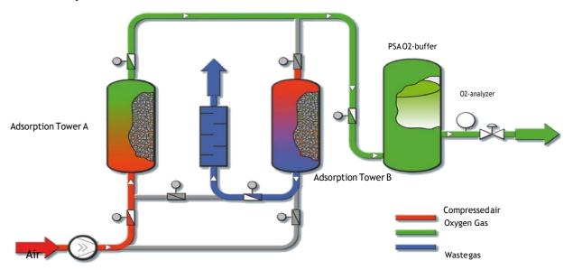
There are two alternately process cycle for PSA Oxygen Generator:
