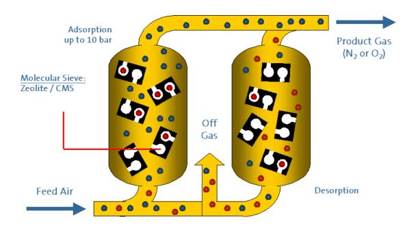
The separation of N2 and O2 from air takes place in an adsorption vessel filled with Zeolite molecular sieve.
